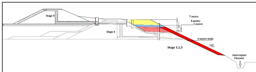
Figure 9: Cross section – facility embankment with buttress
